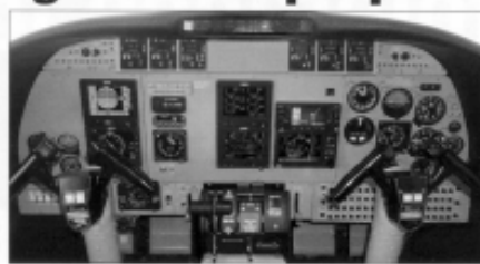
Meggitt's Magic cockpit for Twin Commander includes EFIS and digital flight control.
